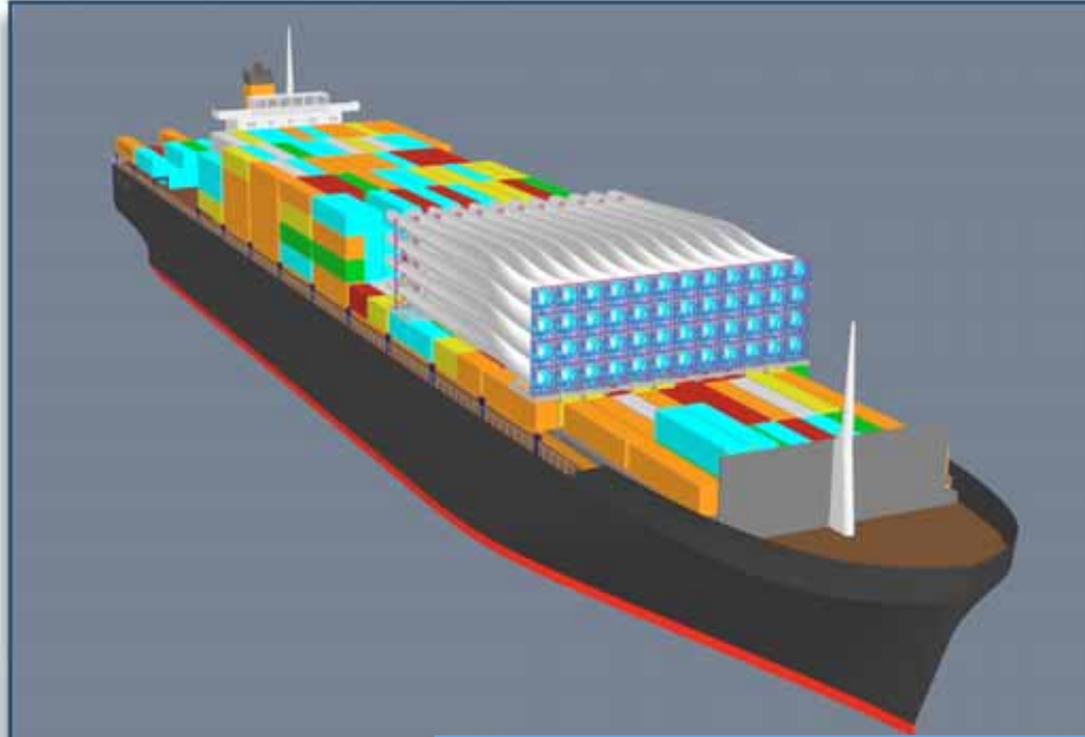
STOWAGE ON 1st. TIER OF 20FT CONTAINER ON PAN MAX OR POSTPAN MAX CONTAINER VESSEL
